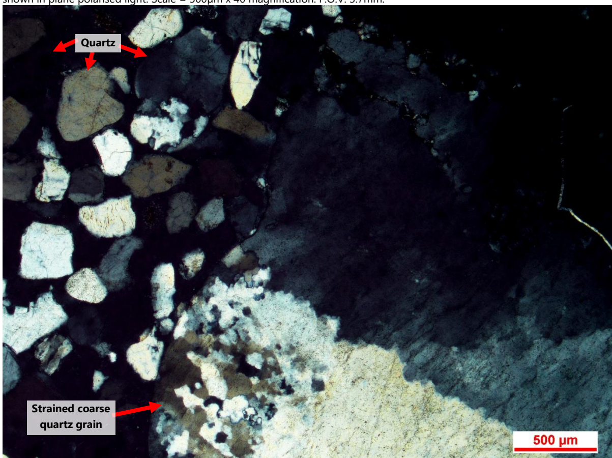
Plate 5: The same image from Plate 4 under crossed polarised light. Scale = 500µm x 40 magnification. F.O.V. 3.7mm.
