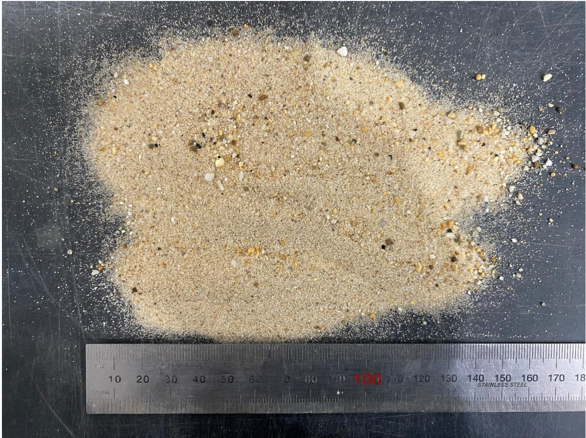
Plate 2: Photograph of the sample as provided, showing the moderately sorted quartz sand.
